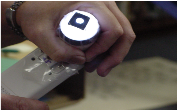
30x lens - The black paper has a 1/4" hole punched in the center. The hole is taped over the center of the lens. A clear plastic sheet is held tightly against the lens.
