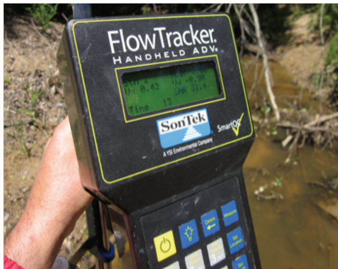
Top: LGS staff conducting a Flow Tracker® survey of Shettleworth Bayou near Shreveport, Louisiana. Botom: A close up view of the Flow Tracker® in operation for survey.
